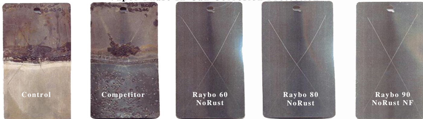
Panels partially immersed in UCAR 379 for 23 days (120°F, pH adjusted to 9.0)
